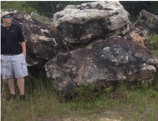
Figure 1: Example of type, size and shape of artificial reef substrate (limestone rip-rap)
