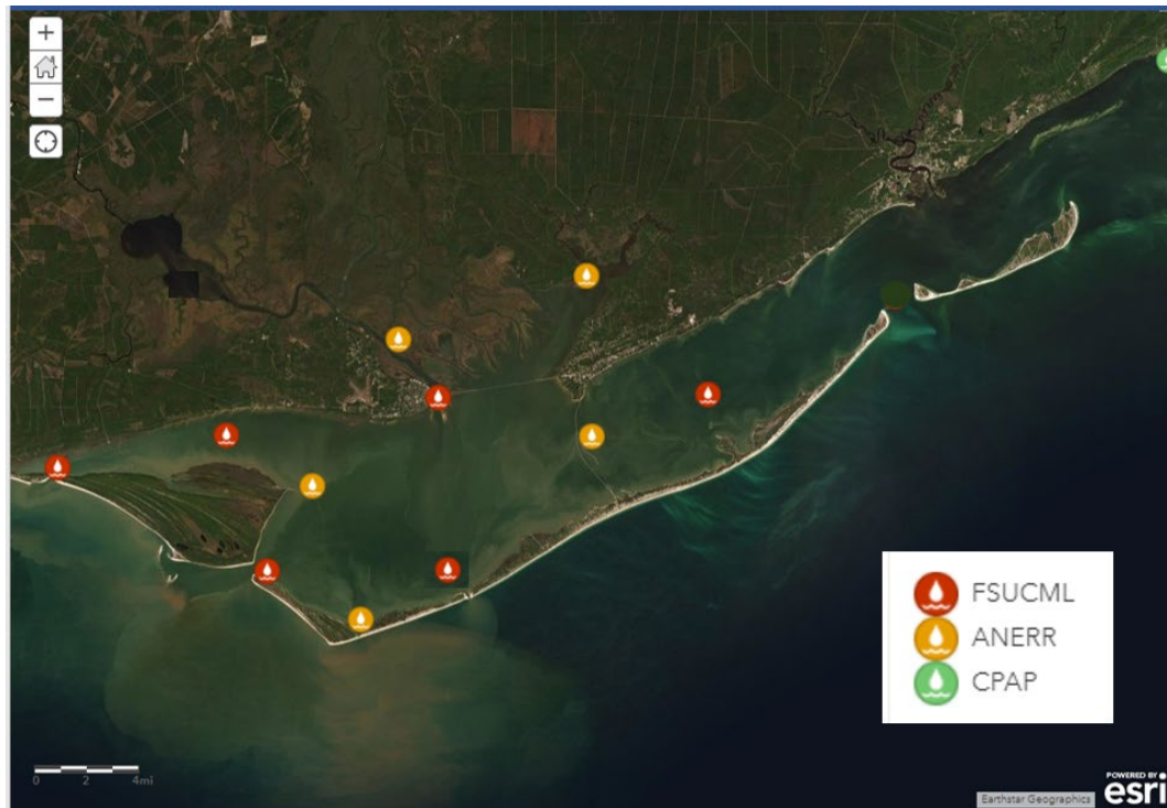
Figure 2. Distribution of instruments (YSI EX02) deployed by the Apalachicola National Estuarine Research Reserve (ANERR), Central Panhandle Aquatic Preserve (CPAP) and ABSI
