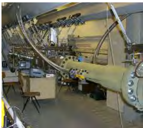
Purdue Mach 6 Quiet Flow Ludwig Tube, 9.5" Diameter Test Section
